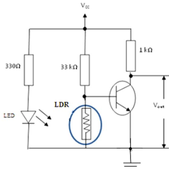
Figure (2) Simple light sensor circuit
