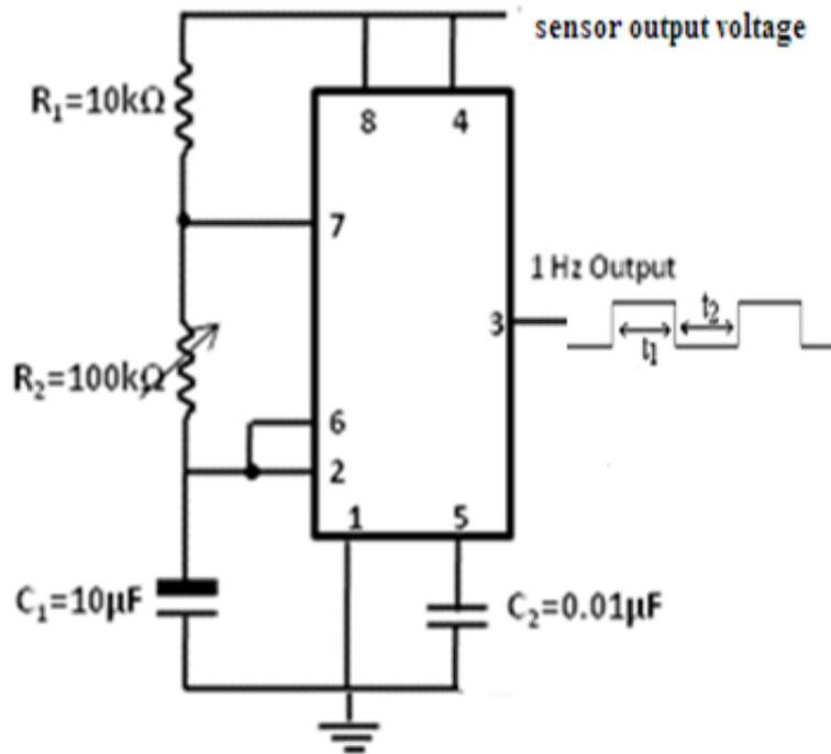
Figure (4) Circuit Diagram of astable operation of 555 Timer IC
