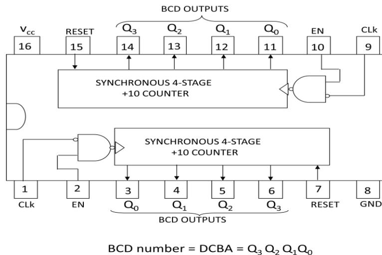
Figure (5) Functional Diagram of 4518B IC
