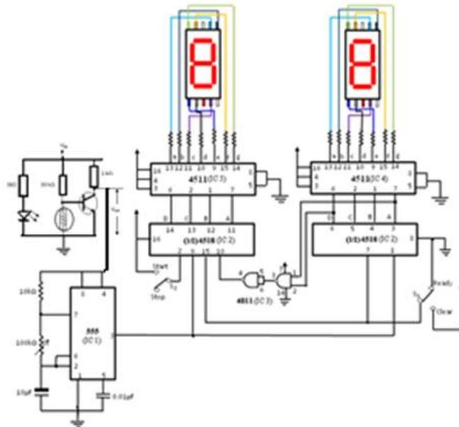
Figure (9) Circuit Diagram of the Whole System
