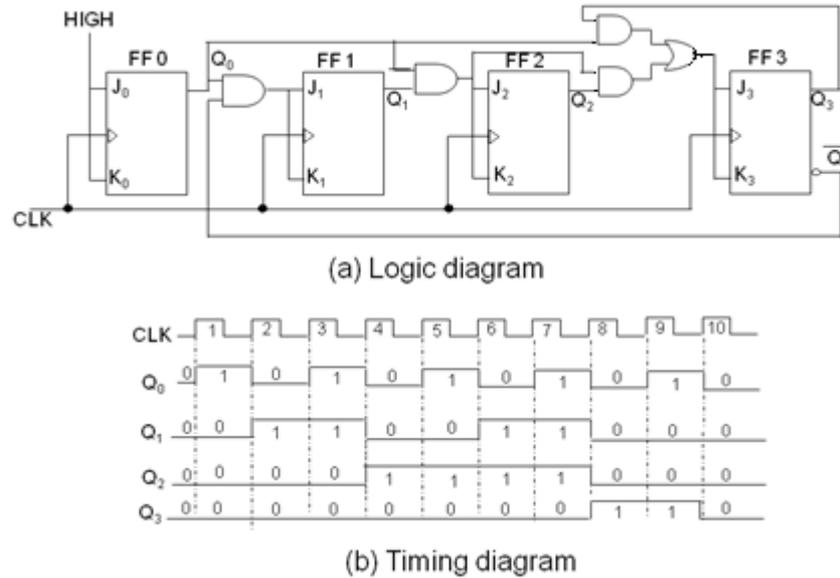
Figure (6) Four bit synchronous decade counter
