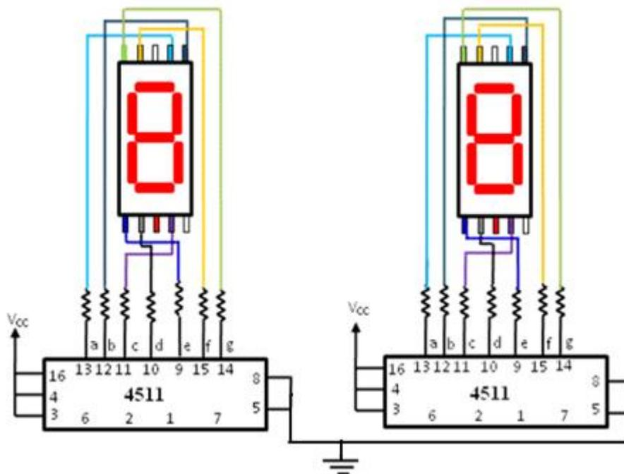
Figure (8) Circuit Design for Display Units Section
