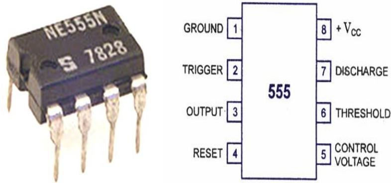
Figure (3) Pin configuration of 555 Timer IC
