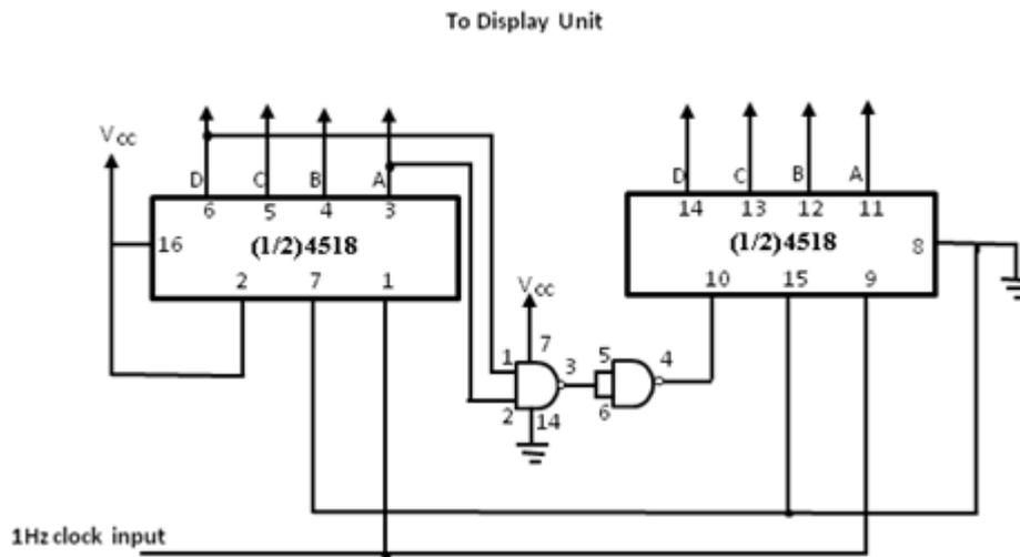
Figure (7) Circuit Design for Counter Section
