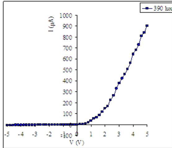
Figure (4-b). I-V characteristic curves of  $\text{Ca}_{0.90}\text{Mg}_{0.10}(\text{CO}_3)_2/\text{n-Si}$  thin film under 390 lux (ambient) illumination condition
