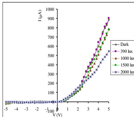
Figure (4-f).Comparison of the I-V characteristic curves of  $\text{Ca}_{0.90}\text{Mg}_{0.10}(\text{CO}_3)_2/\text{n-Si}$  thin film in dark and different illumination conditions
