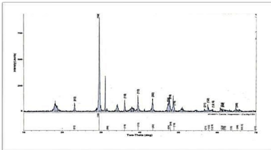
Figure (1) XRD pattern of  $\text{Ca}_{0.90}\text{Mg}_{0.10}(\text{CO}_3)_2$  ceramic
