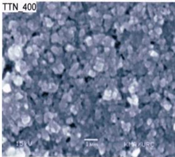
Figure(2) SEM micrograph (surface morphology )  $\text{Ca}_{0.90}\text{Mg}_{0.10}(\text{CO}_3)_2/\text{n-Si}$  thin film.
