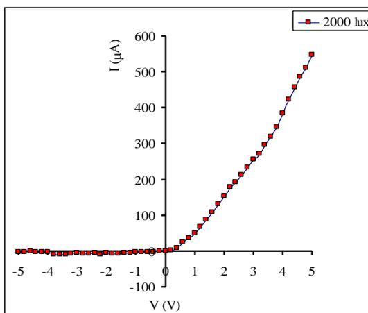
Figure (4-e).I-V characteristic curves of  $\text{Ca}_{0.90}\text{Mg}_{0.10}(\text{CO}_3)_2/\text{n-Si}$  thin film under 2000 lux (ambient) illumination condition
