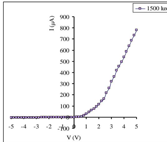
Figure (4-d).I-V characteristic curves of  $\text{Ca}_{0.90}\text{Mg}_{0.10}(\text{CO}_3)_2/\text{n-Si}$  thin film under 1500 lux (ambient) illumination condition
