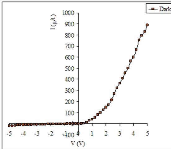
Figure (4-a).I-V characteristic curves of  $\text{Ca}_{0.90}\text{Mg}_{0.10}(\text{CO}_3)_2/\text{n-Si}$  thin film in dark condition
