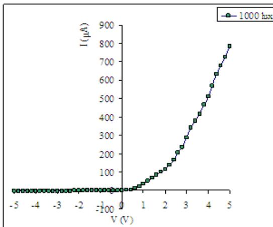
Figure (4-c).I-V characteristic curves of  $\text{Ca}_{0.90}\text{Mg}_{0.10}(\text{CO}_3)_2/\text{n-Si}$  thin film under 1000 lux (ambient) illumination condition
