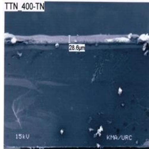
Figure(3) SEM micrograph (diffusion of the layer thickness) of the(top view of the film)  $\text{Ca}_{0.90}\text{Mg}_{0.10}(\text{CO}_3)_2/\text{n-Si}$  thin film (side view of the film)
