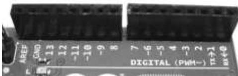
Figure (6) The digital input/output pins
