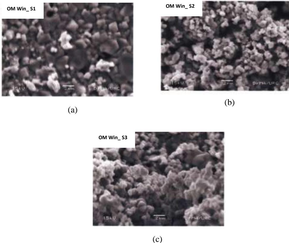
Fig. (4) The SEM micrographs of the sintered surface  $\text{NiFe}_2\text{O}_4$  powder after final sintered at (a)  $1000^\circ\text{C}$ , (b)  $1100^\circ\text{C}$ , (c)  $1200^\circ\text{C}$
