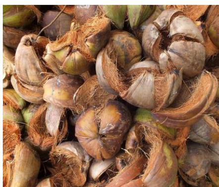
Figure (1) Coconut fruits and coconut husk samples.
