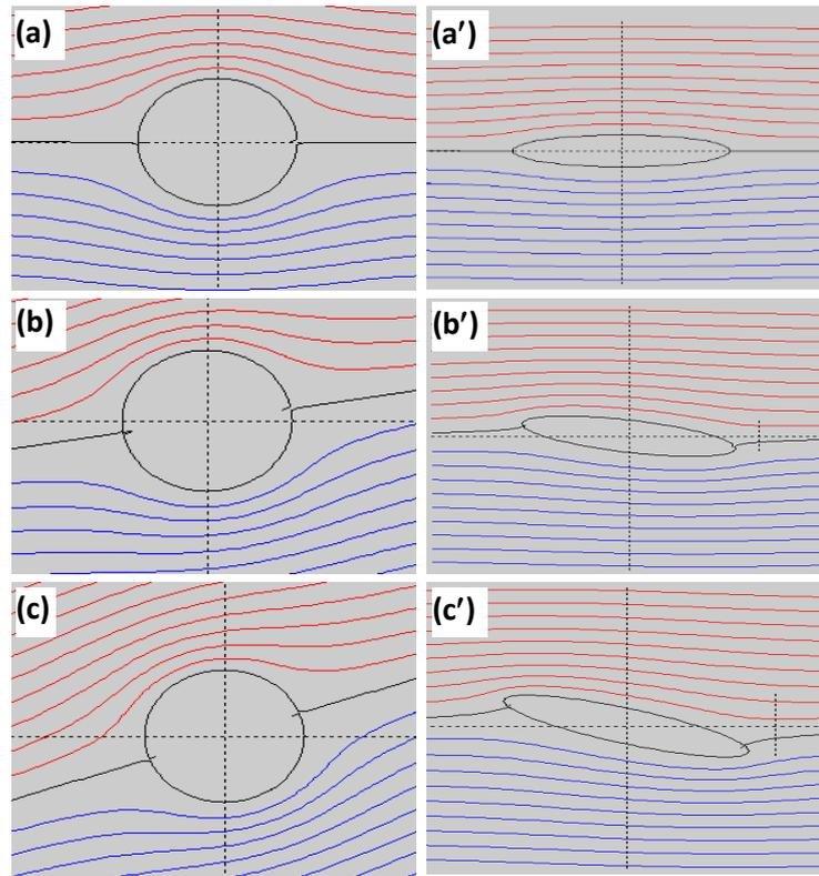
Figure (2). Mapped flow past the circles in Z-plane (Figures a, b, and c) to the flow past an ellipse the z-plane (Figures a', b', and c').
