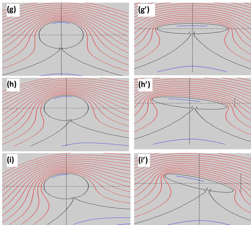
Figure (4). Mapped circulation flow past the circles in Z-plane (Figure g, h, and i) to the flow past an ellipse the z-plane (Figures g', h', and i').
