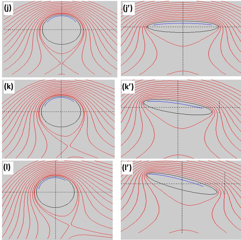
Figure (5). Mapped circulation flow past the circles in Z-plane (Figures j, k, and l) to the flow past an ellipse the z-plane (Figures j', k', and l').
