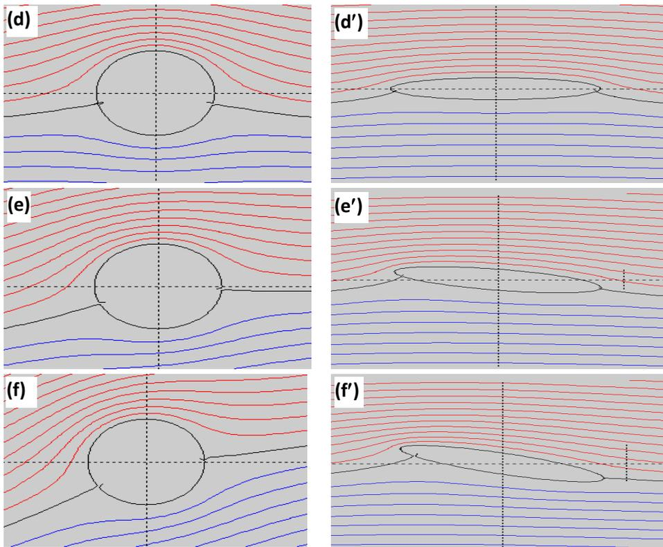
Figure (3). Mapped circulation flow past the circles in Z-plane (Figures d, e, and f) to the flow past an ellipse the z-plane (Figures d', e', and f').
