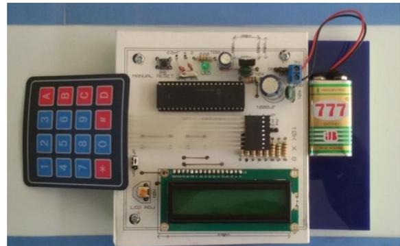
Figure (9). The photograph of PIC 16F887 based integer calculator circuit
