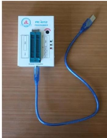
Figure (7). The photograph of programmer circuit board
