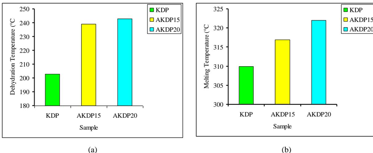
Figure (6). Comparison of the (a) dehydration temperatures and (b) melting temperatures of the KDP, AKDP15 and AKDP 20 crystals.
