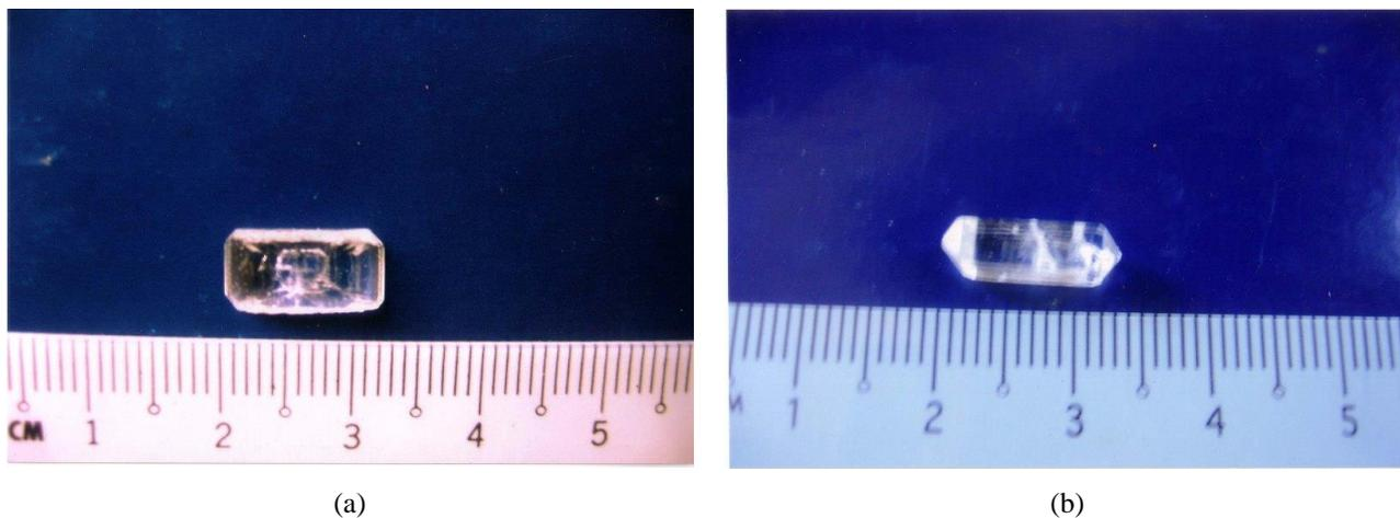
Figure (1). Photographs of the as-grown (a) AKDP15 and (b) AKDP20 crystals.
