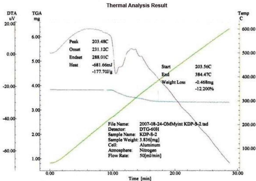
Figure (5). TG-DTA thermograms of KDP crystal.
