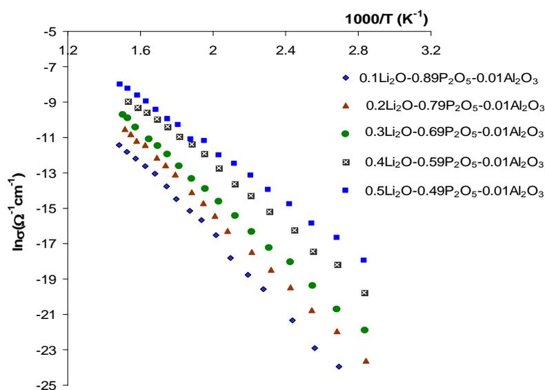
Figure 4 The result for temperature dependent conductivity measurement on yLi<sub>2</sub>O. (0.99-y) P<sub>2</sub>O<sub>5</sub>. 0.01 Al<sub>2</sub>O<sub>3</sub> glasses
