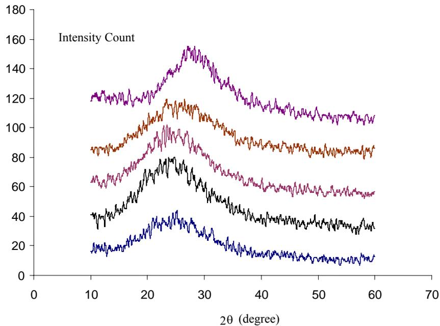
Figure 2 XRD Pattern for  $y\text{Li}_2\text{O} \cdot (0.99-y)\text{P}_2\text{O}_5 \cdot 0.01\text{Al}_2\text{O}_3$  Glasses
