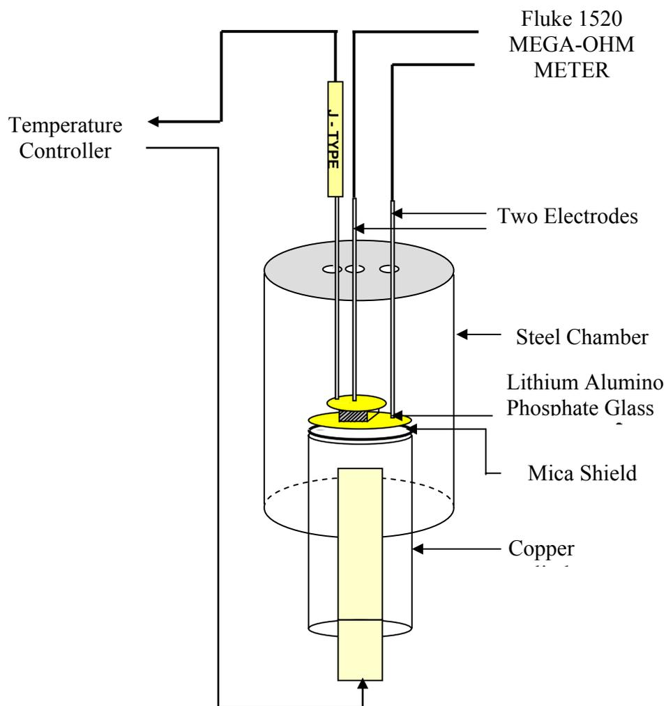
Figure 3 Experimental arrangements for conductivity measurement
