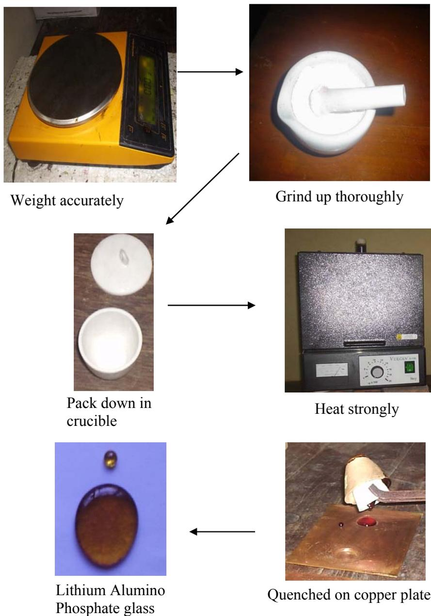
Figure 1 Reaction scheme for the formation of Lithium Alumino Phosphate glasses using the melt-quenching method.
